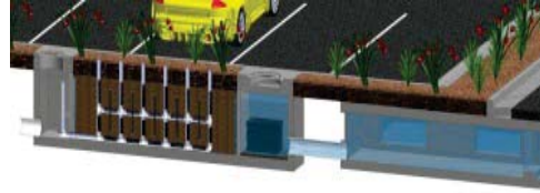
Horizontal Flow Biofiltration System
